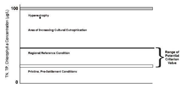
**Figure 1-5.** Derivation of the reference condition and the National Nutrient Criteria Program using TP, TN, and chlorophyll *a* as example variables. Clarity or Secchi depth would be on a reversed scale. Protectivity nutrient criteria should be between pristine conditions and present reference conditions, i.e., the most "natural" attainable.
